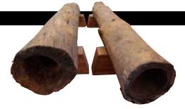
Seen in the photo are sections of wooden piping on display at the sanatorium's museum. Made from Japanese red pine, they are approximately 40 centimeters in diameter and 180 centimeters long. Patients were involved in the work of hollowing out the logs, which were laid end to end and buried in the earth.
